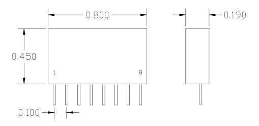
Pin 1 is Input Pin 8 is Output Pins 2 thru 7 are Ground
